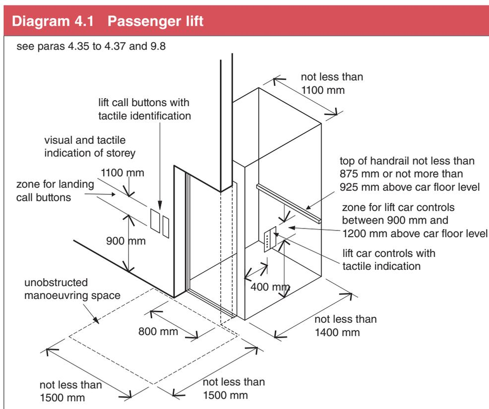
A passenger lift should have a power operated horizontal sliding door or doors which provide a clear width of not less than 800 mm. See Diagram 4.1.
